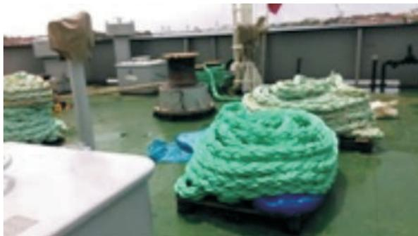
**Figure no. 3.11 Mooring lines on deck**
